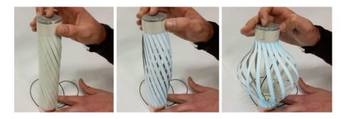
Fig. 2 - The demonstrator features a dimming effect corresponding to structural deformation
