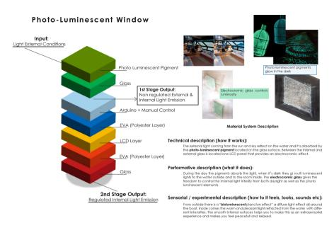
Fig. 4 - Glowrious smart windows material graphical schematic representation on the Concept Canvas
